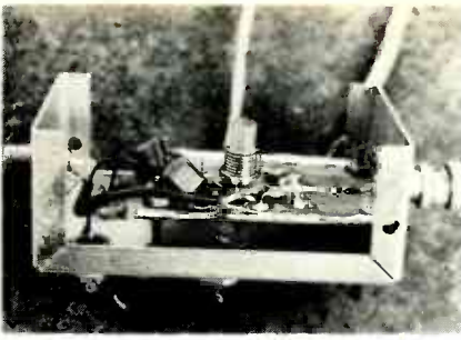
ACTIVE MIXER USING HFET device along with VTO 8360 (mounted out of sight on back side) mounts in single container. Unit can mount outside, at antenna, if appropriately weather-proofed thereby running only 70-MHz IF energy down and inside (in low-cost 50- or 75-ohm coaxial cable).
